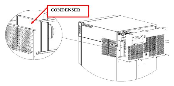
Figure 23 - Condenser position in models 100-140-280
