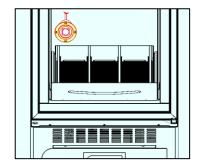
Figure 16 – position of the SUPERARTIC model pressure equalising valve
