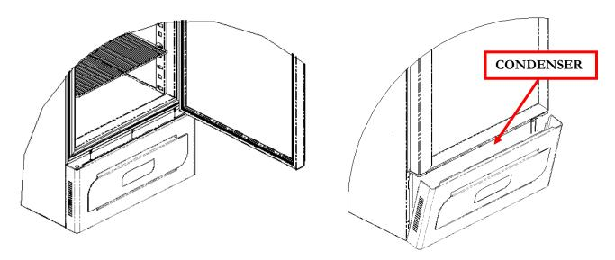
Figure 24 - Condenser position in models with lower compartment motor
