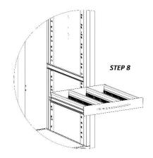
Figure 10 – installation of drawer on rack
