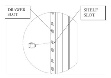
Figure 5 – Slots for internal fittings
