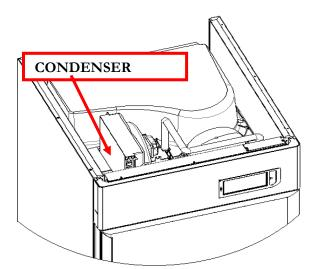
Figure 25 - Condenser position in models 700-1500
