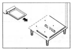
Figure 27 - Tray with automatic condensate water evaporation
