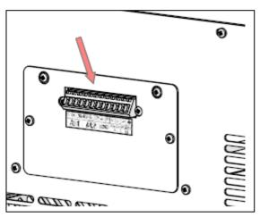
Figure 21 - Position of the terminal board for alarm relay
