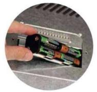
Figure 20 - Buffer batteries
