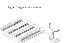
Figure 9 - installation of guides on drawer
