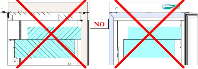
Figure 13 – INCORRECT material storage
