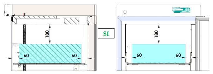
Figure 12 – Correct material storage
